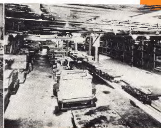
In this die storage department are more than 5,000,000 pounds of dies used in building Oliver "Cletrac" tractors. Dies are handled and stored electrically.
