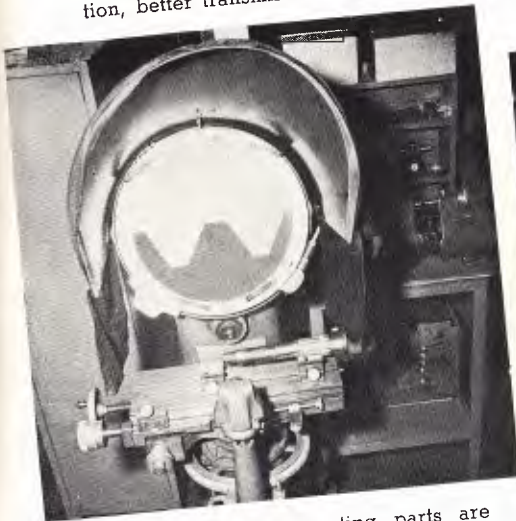
All machined and operating parts are checked by the highest standard gauges known. But to insure accuracy of fit of all parts, templates and thread contours are magnified 62½ times.
