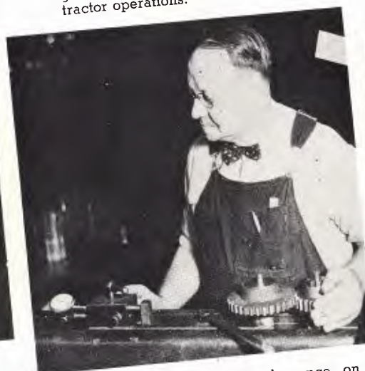
Correct "back lash," or clearance on making gears is constantly checked on the finest of precision equipment. The result is smooth, efficient power transmission.
