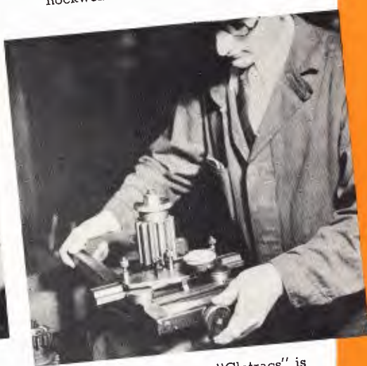
The building of Oliver "Cletracs" is a constant check, check and double check. This gear testing instrument registers in ten-thousandths of an inch.
